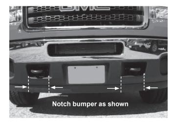
Beginning with the passenger-side mount, align the forward mount holes with tow hook holes in frame. Reinstall the tow hook and fasteners and tighten according to the torque charts provided. Repeat on the opposite side.
