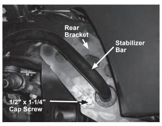
4. Insert a 1/2" x 1-3/4" cap screw and washer through the rectangular opening in the inner surface of the frame, through the frame and the rear bracket. Secure loosely with a 1/2" locknut. Adjust the position of the rear brackets upwards as far as possible and secure the 1-3/4" fastener, as well as the three 1-1/4" cap screws from step 3.
