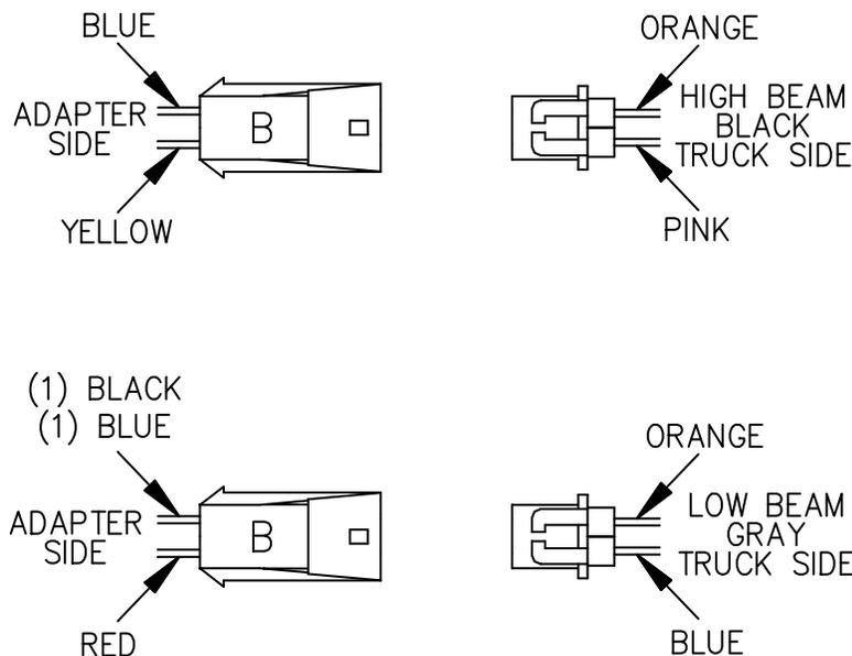
**Figure 1.** Headlight Adapter Orientation
