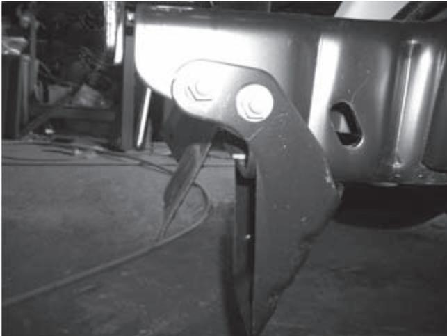
3. Remove the metal sway bar brackets and retain for reinstallation later in this procedure.
